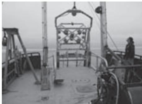
Camera sled being deployed south of St. Lawrence Island.
